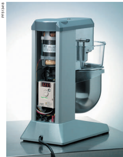
ATV12 controlling a mixer
